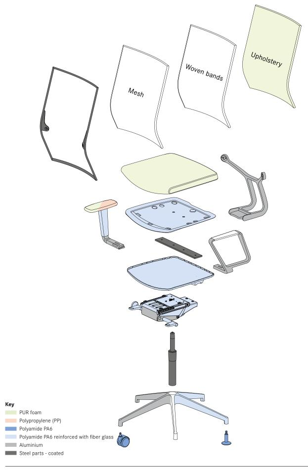
The way in which Diagon is constructed allows the chair to be dismantled at the end of its working life in order to recycle most of the parts. A detailed list of the materials used follows:
