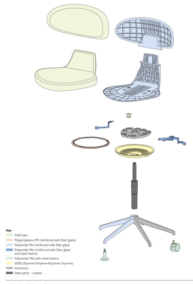
The way in which Simplex 3D is constructed allows the chair to be dismantled at the end of its working life in order to recycle most of the parts. A detailed list of the materials used follows:
