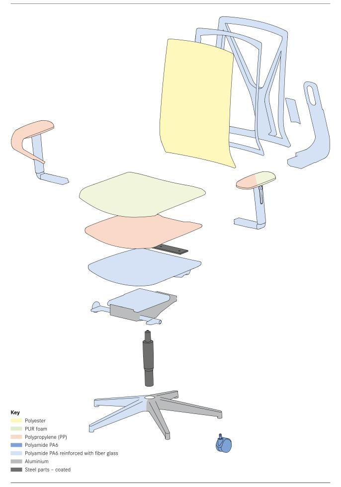
The way in which Yanos is constructed allows the chair to be dismantled at the end of its working life in order to recycle most of the parts. A detailed list of the materials used follows:
