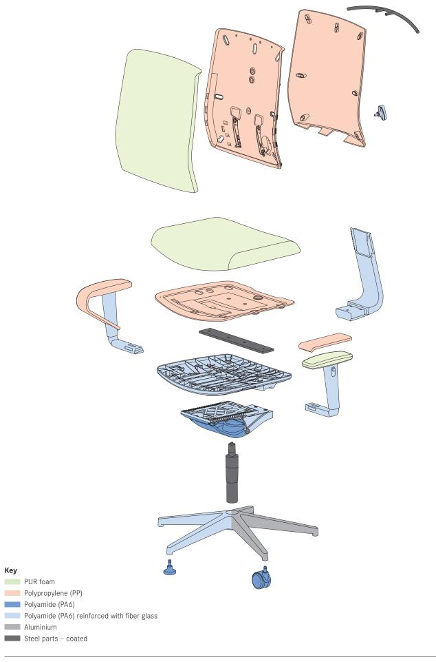
The way in which Kyra Flex is constructed allows the chair to be dismantled at the end of its working life in order to recycle most of the parts. A detailed list of the materials used follows:
