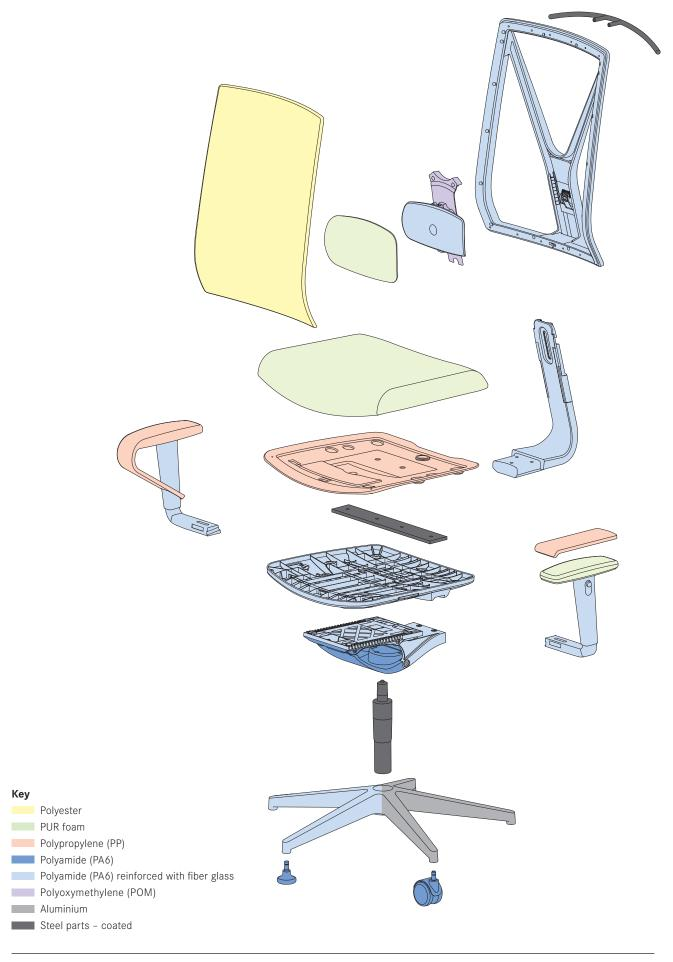
The way in which Yanos Flex is constructed allows the chair to be dismantled at the end of its working life in order to recycle most of the parts. A detailed list of the materials used follows:
